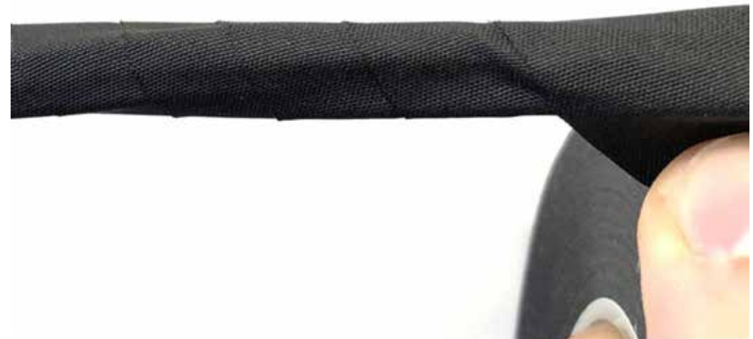
Use the roll close to the harness with a constant, tight winding and a triple final layer
